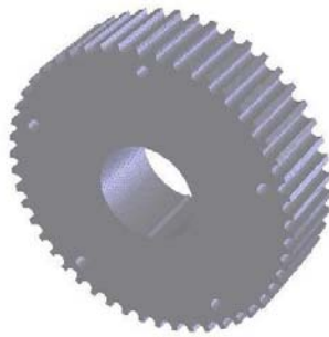
Rotor Lamination Stack – 21 pieces stamped from 0.5mm silicon iron sheet.
